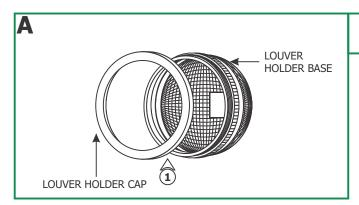
1: Unscrew and remove the louver holder cap from the louver holder base.
