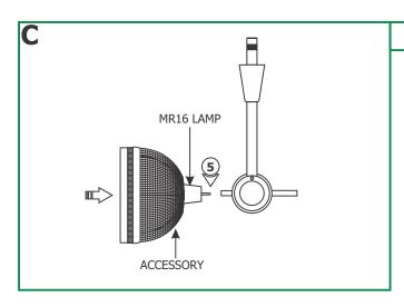
5: Push the lamp pins completely into the socket holes.
