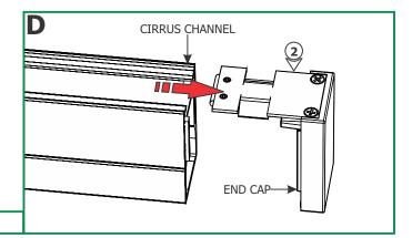
2: Slide the end cap out of the channel.
