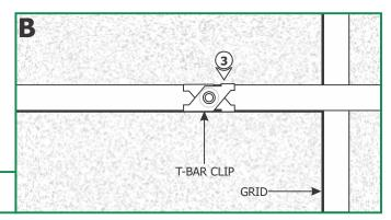
**3:** Place the T-Bar clip onto the grid and squeeze the arms together to secure it in place.
