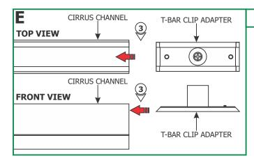
**4:** Align the T-bar clip adapters evenly apart and tighten the #6-32 set screws on each T-bar clip adapter with a 1/16" Allen wrench.
