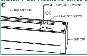
**1:** Loosen the two #4-40 set screws (**DO NOT REMOVE**) on the end cap at the non-power side of the Cirrus channel using a 0.05" Allen wrench.
