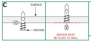
**NOTE:** Steps 5 and 6 are for drywall mounting. Omit these steps if mounting the clips to a wood surface directly.
