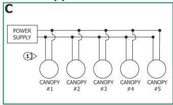
1: Insert the power supply (TE-60L-12) into an electrical box to branch the power to each Fast Jack canopy. The power supply wires are connected in parallel with Fast Jack canopy wires. It is recommended to install each canopy near the power supply to avoid voltage drop. Refer to the chart below for the proper low voltage wire size.
