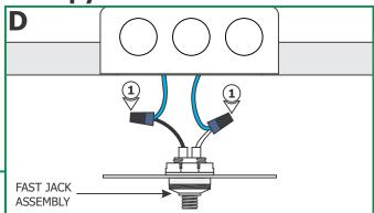
**1:** Connect each Fast Jack assembly wire to one low voltage transformer wire with a wire nut.
