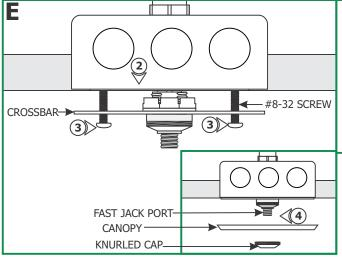
2: Place all wire nut connections inside the electrical box.
