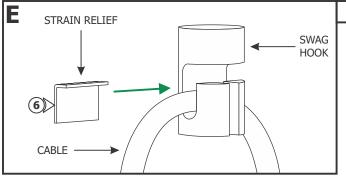
**6:** Insert the strain relief into the swag hook behind the cable.
