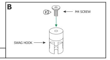
**2:** Insert the M4 screw halfway into the swag hook using a 2.5mm Allen wrench.
