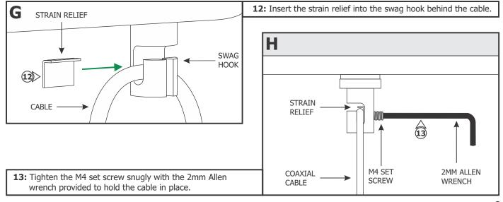
11: Slide the coaxial cable into the swag hook through the center opening or the side opening. If necessary, rotate the bracket
