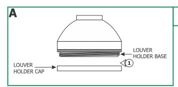
1: Unscrew and remove the louver holder cap from the louver holder base.
