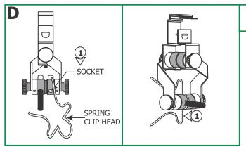
**1:** Push the spring clip completely onto the center of the socket groove until it snaps into place.
