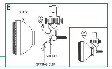
**2:** Squeeze the spring clip ends while inserting it into the shade.
