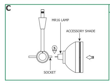
5: Push the lamp pins completely into the socket holes.
